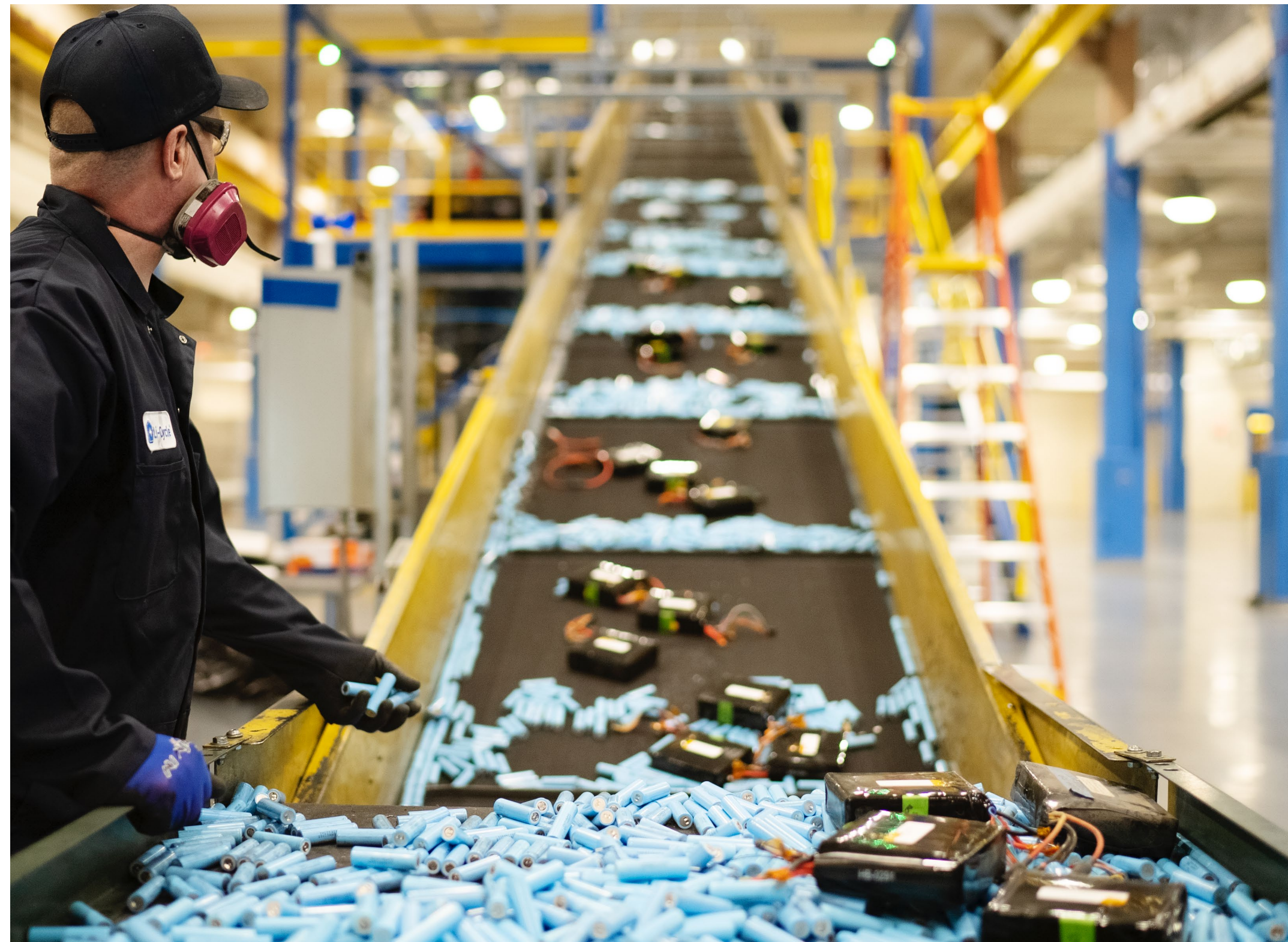
Li-Cycle employee feeds lithium-ion batteries on conveyor belt inside one of the company's Spoke facilities
